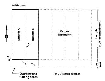
Figure 1. Common bunker silo arrangement.
