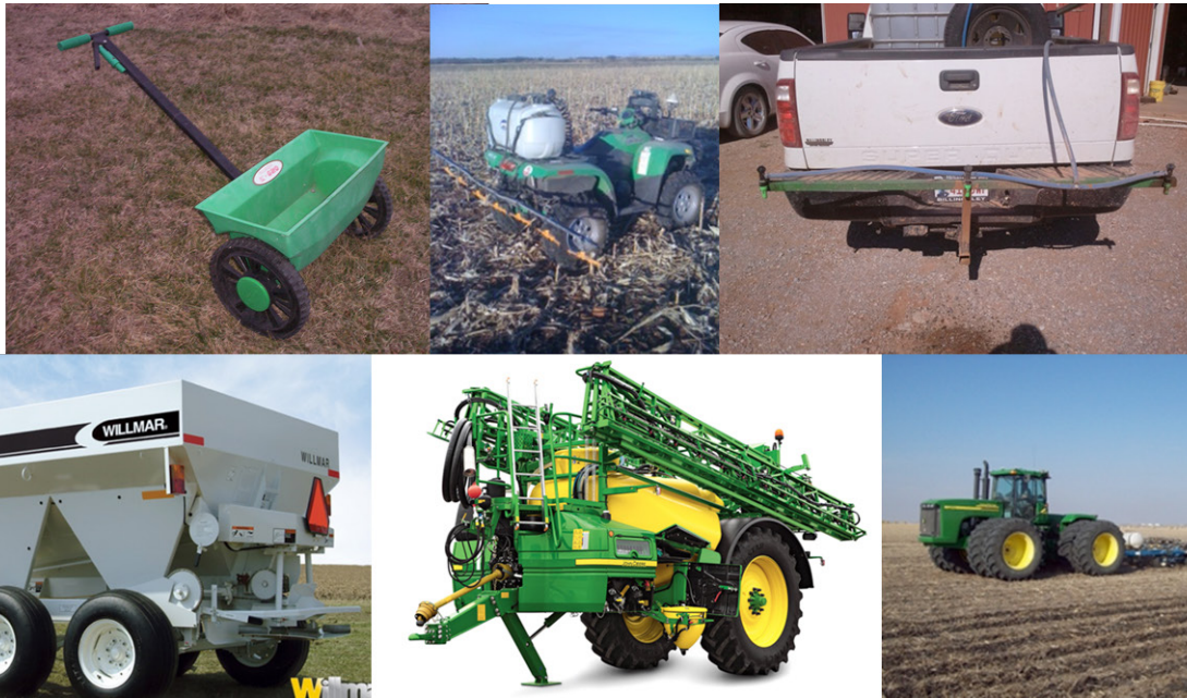
Figure 2. Equipment used for N-Rich Strips. From top-left to bottom right: Push spreader, ATV with 10-foot spray boom, receiver hitch mount with trigger in cab, dry fertilizer spreader, sprayer pull or self-propelled (often only use middle section) and anhydrous applicator.
