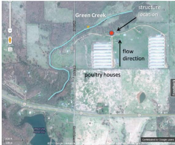
This confined bed filter contained 40 tons of sieved and treated steel slag. The structure was designed to remove 45 percent of the estimated annual DP load (20 lbs) and handle flow rates from a two-year/24 hour storm (16 cfs).
