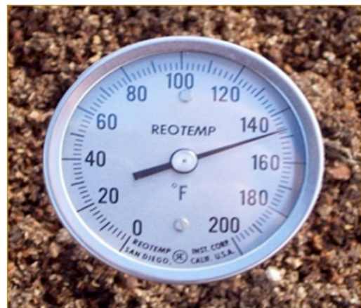
Figure 6. Long-stem thermometer used to monitor temperature.
