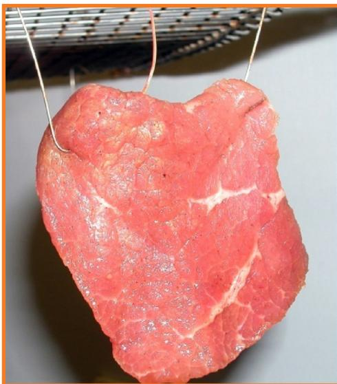
Figure 1. Beef jerky hanging in a dehydrator from two wire hooks (thermocouple wire is visible in top center of photo).
