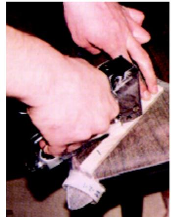
Figure 6F. Staple larger wood lath to inside of cone.
