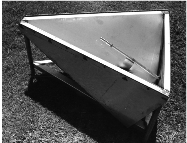
Figure 3. Inclined stainless steel pressure rinse/drain rack.
