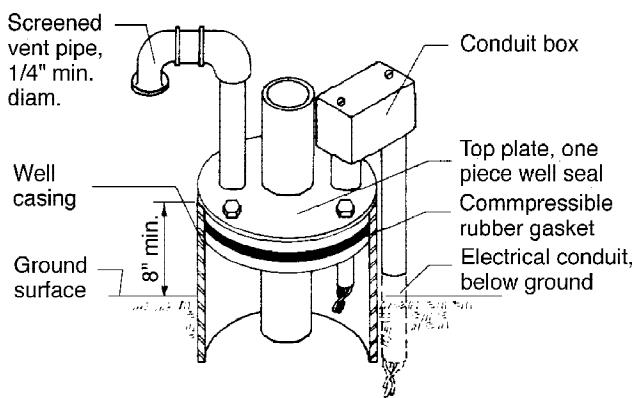
Figure 2. A sanitary well seal with screened vent pipe to protect a water well from surface water, vermin and foreign matter.
