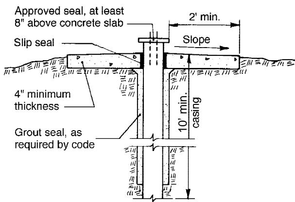
Figure 1. Recommended construction for water wells to protect the ground water supply from contamination.
