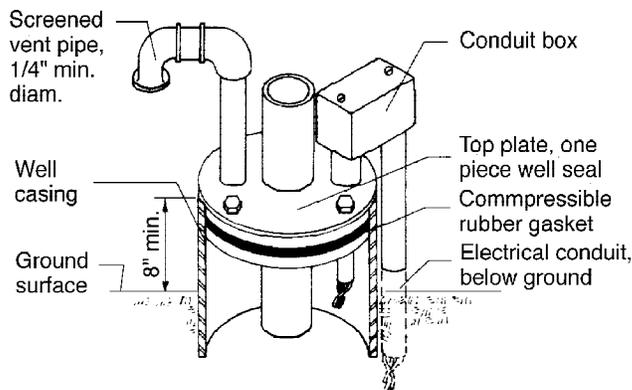
**Figure 2.** A sanitary well seal with screened vent pipe to protect a water well from surface water, vermin and foreign matter.
