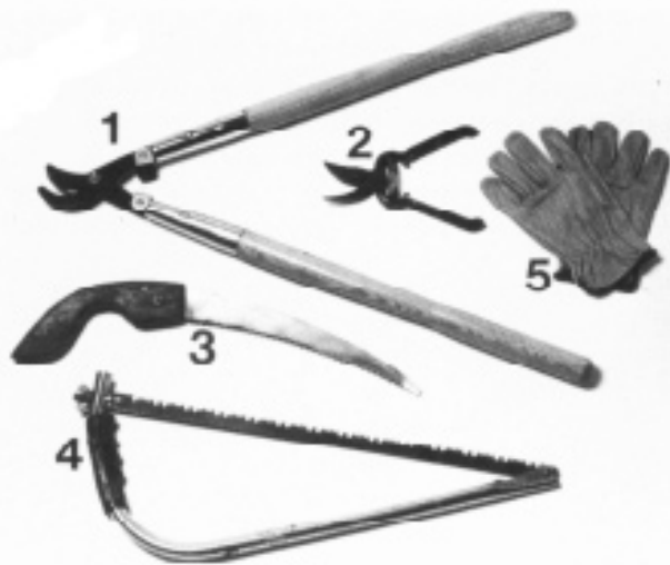
Figure 1. (1) lopping shear (2) hand pruner (3) folding saw for tight places (4) bow saw for limbs and (5) leather gloves. Note, carpenters saws gum up, pruning saws do not.
