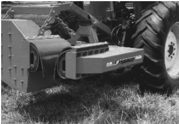
Figure 2. A Pecan Shaker Equipped with Donut Pads.
